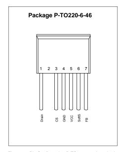
Figure 3 Pin Configuration P-TO220-6-46(top view)
