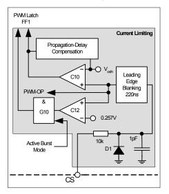
Figure 12 Current Limiting Block
