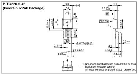
Figure 23 P-TO220-6-46 (Isodrain I2Pak Package)
