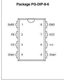
Figure 1 Pin Configuration PG-DIP-8-6(top view)
