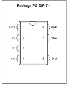
Figure 2 Pin Configuration PG-DIP-7-1(top view)
