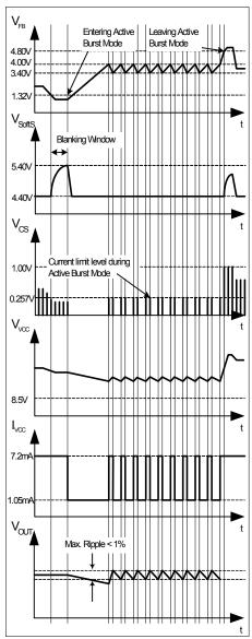
Figure 19 Signals in Active Burst Mode
