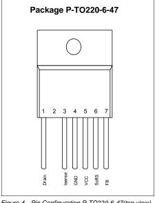
Figure 4 Pin Configuration P-TO220-6-47(top view)
