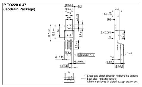
Figure 24 P-TO220-6-47 (Isodrain Package)
