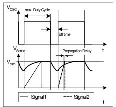
Figure 16 Dynamic Voltage Threshold V<sub>csth</sub>
