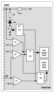
Figure 17 Adjustable Blanking Window
