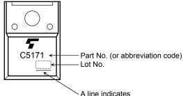
A line indicates lead (Pb)-free package or lead (Pb)-free finish.
