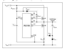
Figure 1, Start-up and supply circuitry.
