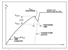
Figure 2, Supply capacitor (CVCC) voltage.
