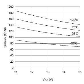
Graph 24.  $t_{RISE(HO)}$  vs  $V_{CC}$  vs Temperature (IR2156)
