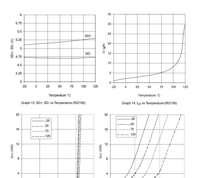
Graph 15. IQCC vs VCC vs Temperature (IR2156)
