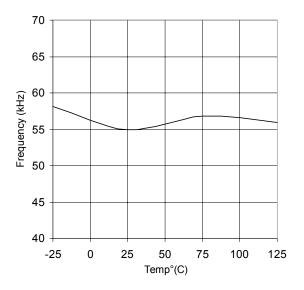
Graph 20.  $F_{OSC}$  vs Temperature (IR2156)  $V_{CPH} = 0V$
