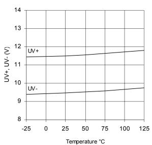
Graph 11. R<sub>VDC</sub>+ vs Temperature (IR2156)
