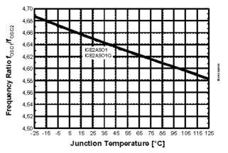
Figure 34 Frequency Ratio  $f_{OSC1}/f_{OSC2}$  vs.  $T_j$
