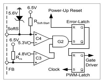
Figure 10 Activation of Protection Unit
