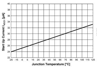
Figure 23 Start Up Current  $I_{VCC1}$  vs.  $T_j$
