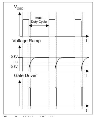
Figure 7 Light Load Conditions
