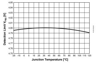
Figure 40 Detection Limit  $V_{FB2}$  vs.  $T_j$
