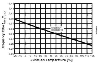
Figure 35 Frequency Ratio  $f_{OSC3}/f_{OSC4}$  vs.  $T_j$
