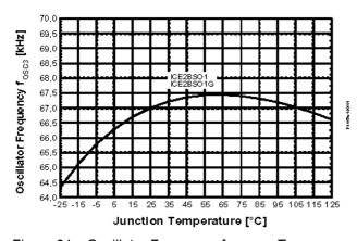
Figure 31 Oscillator Frequency  $f_{OSC3}$  vs.  $T_j$
