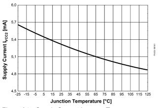
Figure 24 Supply Current  $I_{VCC2}$  vs.  $T_i$
