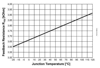
Figure 38 Feedback Resistance  $R_{FB}$  vs.  $T_j$
