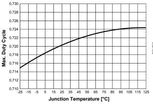
Figure 36 Max. Duty Cycle vs. T<sub>i</sub>
