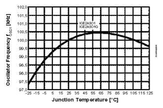
Figure 30 Oscillator Frequency  $f_{OSC1}$  vs.  $T_i$
