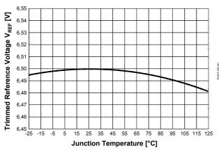
Figure 29 Trimmed Reference  $V_{REF}$  vs.  $T_i$
