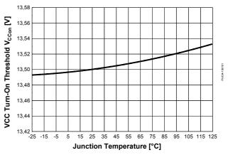
Figure 26 VCC Turn-On Threshold  $V_{VCCon}$  vs.  $T_j$
