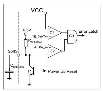
Figure 22 Overvoltage Detection
