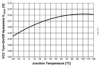
Figure 28 VCC Turn-On/Off Hysteresis  $V_{VCCHY}$  vs.  $T_i$
