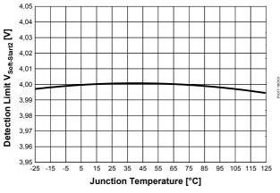
Figure 42 Detection Limit V<sub>Soft-Start2</sub> vs. T<sub>i</sub>
