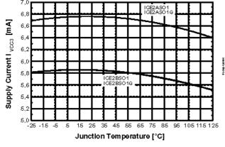
Figure 25 Supply Current  $I_{VCC3}$  vs.  $T_i$
