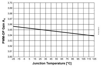
Figure 37 PWM-OP Gain  $A_V$  vs.  $T_j$
