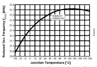
Figure 32 Reduced Osc. Frequency  $f_{OSC2}$  vs.  $T_j$
