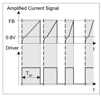
Figure 5 Pulse Width Modulation
