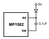
Figure 2—External Bootstrap Diode
