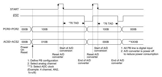
Note: "\*" A/D converting time is 76 TAD
