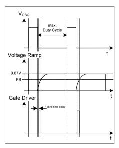
Figure 7 Light Load Conditions
