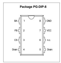
Figure 1 Pin Configuration PG-DIP-8 (top view)
