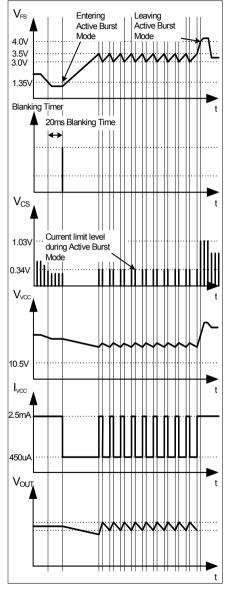
Figure 24 Signals in Active Burst Mode
