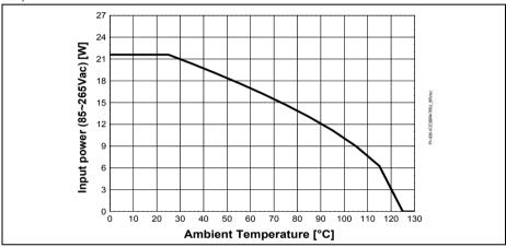
Figure 31 Input power curve Vin=85~265Vac;  $P_{in}$ =f( $T_a$ )
