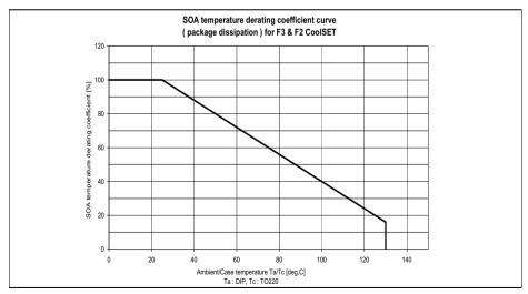
Figure 28 SOA temperature derating coefficient curve
