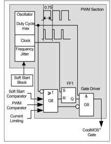
Figure 14 PWM Section Block
