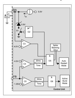
Figure 22 Basic and Extendable Blanking Mode
