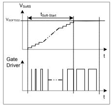
Figure 12 Gate drive signal under Soft-Start Phase
