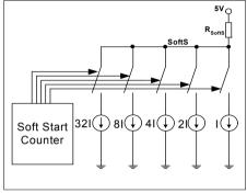
Figure 11 Soft Start Circuit
