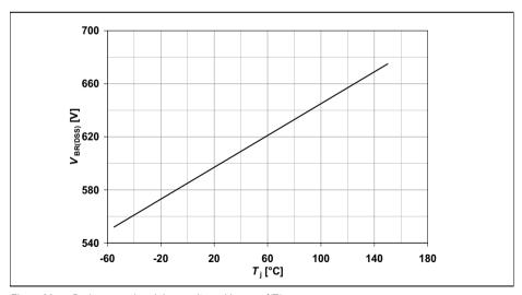
Figure 30 Drain-source breakdown voltage;  $V_{BR(DSS)}$ = $f(T_i)$
