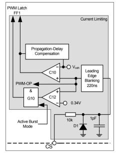
Figure 17 Current Limiting Block
