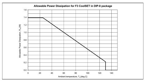
Figure 29 Power dissipation;  $P_{tot}$ = $f(T_a)$
