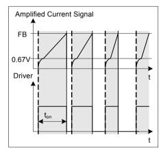
Figure 5 Pulse Width Modulation
