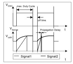
Figure 21 Dynamic Voltage Threshold V<sub>csth</sub>
