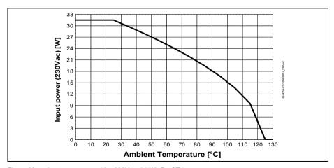
Figure 32 Input power curve Vin=230Vac+/-15%;  $P_{in}$ =f( $T_a$ )
