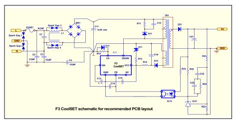
Figure 35 Schematic for recommended PCB layout
