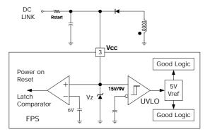
Figure 1. Undervoltage lockout (UVLO) circuit
