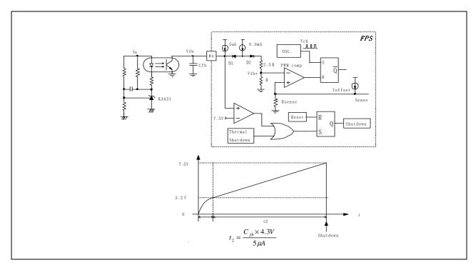
Figure 3. Pulse-width-modulation (PWM) block
