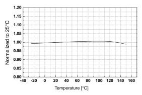
Figure 11. SoftStart Voltage vs. Temp.
