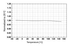
Figure 3. Start Threshold Voltage vs. Temp.
