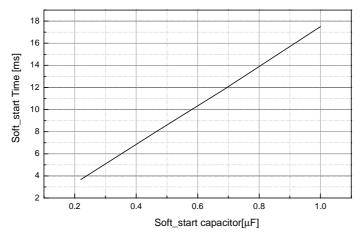
Figure 15. Soft\_start Capacitor vs. Soft\_start Temp.
