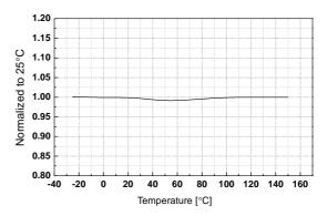
Figure 4. Stop Threshold Voltage vs. Temp.
