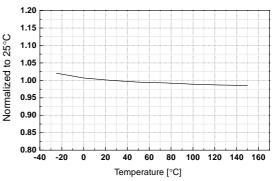
Figure 12. Over Voltage Protection vs. Temp.
