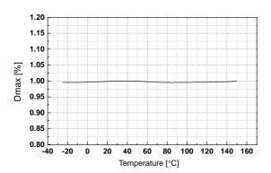
Figure 6. Maximum Duty Cycle vs. Temp.
