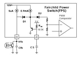
Figure 5. Soft Start Circuit
