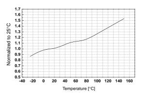
Figure 8. Feedback Offset Voltage vs. Temp.
