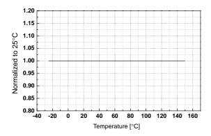
Figure 7. Minimum Duty Cycle vs. Temp.
