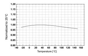
Figure 1. Operating Supply Current vs. Temp.
