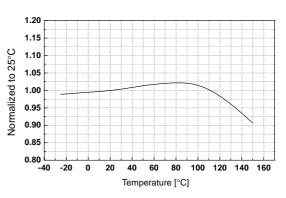
Figure 10. Shutdown Delay Current vs. Temp.
