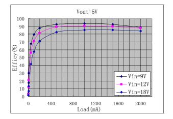
Figure 2. Typical Efficiency Curve
