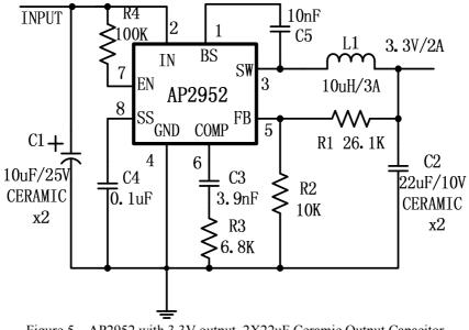
Figure 5 AP2952 with 3.3V output, 2X22uF Ceramic Output Capacitor
