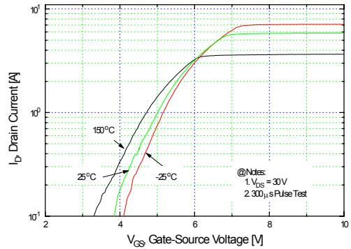
**Figure 2. Transfer Characteristics**
