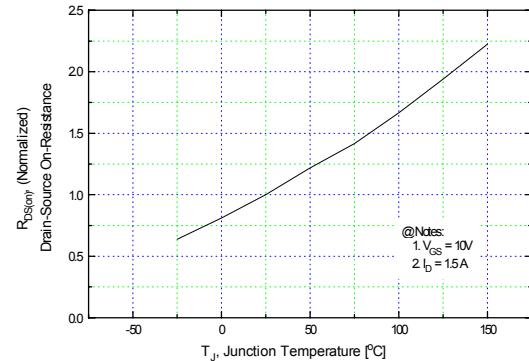
**Figure 8. On-Resistance vs. Temperature**
