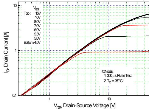
**Figure 1. Output Characteristics**
