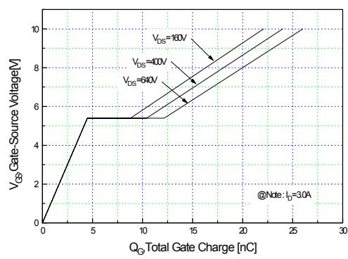
**Figure 6. Gate Charge vs. Gate-Source Voltage**
