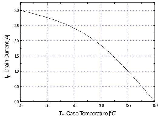
**Figure 10. Max. Drain Current vs. Case Temperature**
