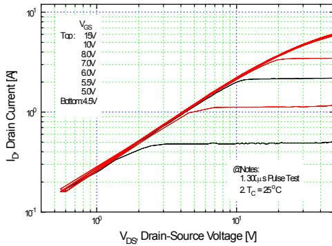
**Figure 1. Output Characteristics**
