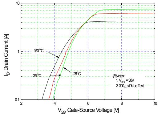
**Figure 2. Transfer Characteristics**
