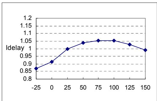
**Figure 11. Shutdown Delay Current**
