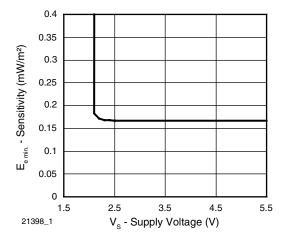
Fig. 13 - Sensitivity vs. Supply Voltage
