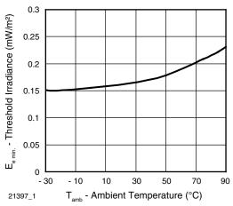
Fig. 10 - Sensitivity vs. Ambient Temperature
