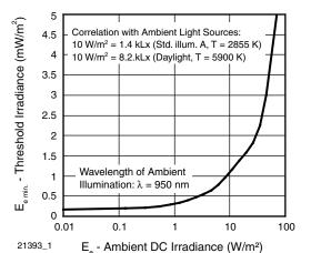
Fig. 6 - Sensitivity in Bright Ambient
