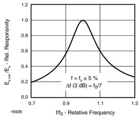
Fig. 5 - Frequency Dependence of Responsivity
