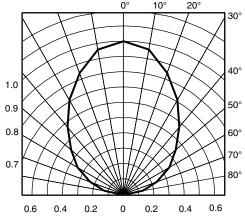
$d_{rel}$  - Relative Transmission Distance Fig. 12 - Horizontal Directivity
